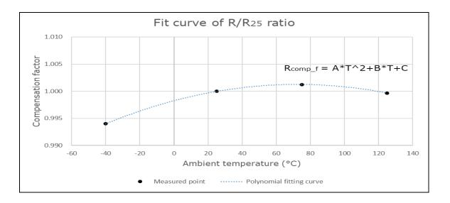
Generic compensation factor the resistance of shunt need to be multiplied with:
